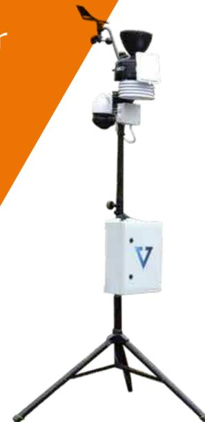
**A complete set for remote controlled operations with multiple applications.**
